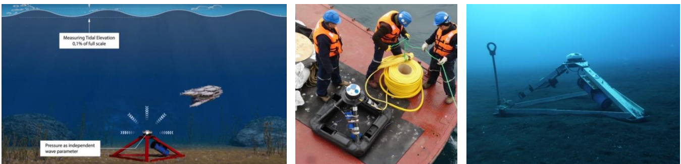
Figure 14: AWAC system for measuring tidal variation or infragravity waves.
