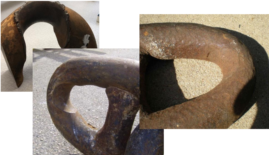
Interlink wear in mooring chains
