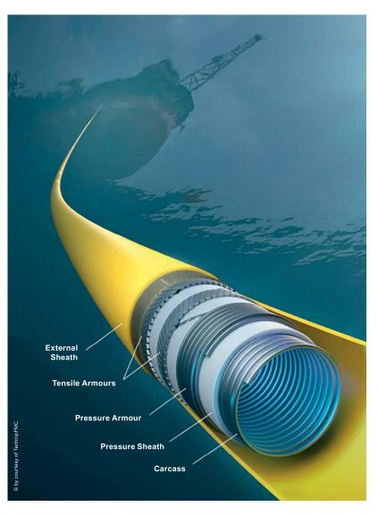
Small-scale tests and full-scale tests are performed to determine material properties and qualify the materials for pressure sheath and outer sheath versus their actual environment while considering relevant interactions with the other layers (pipe body and end-fitting area).
