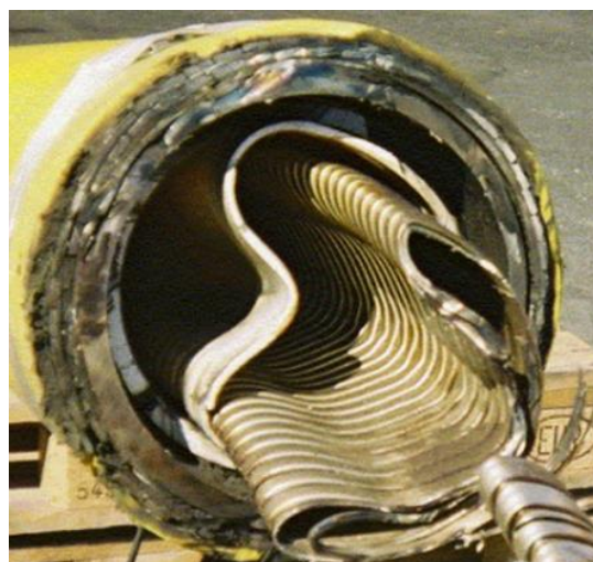
Picture of a collapsed carcass from [SEAFLEX, The Petroleum Safety Authority Norway]
