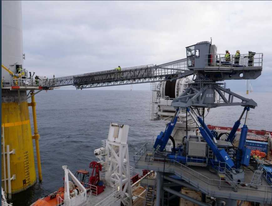
SOV, walk2work, Hywind Tampen (motion compensated gangway)
